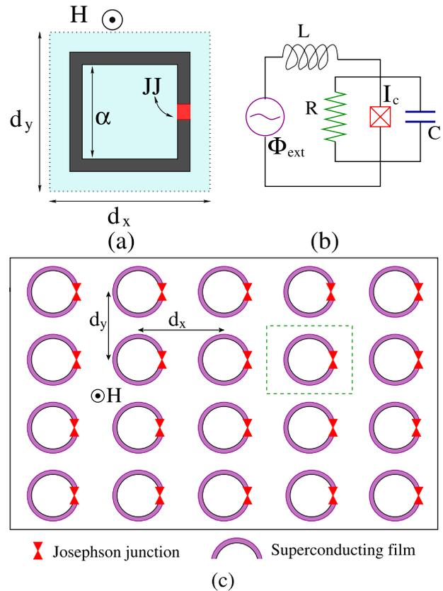
**Figure 1.** (a) Schematic drawing of an rf SQUID in a perpendicular time-dependent magnetic field  $H(t)$ . (b) Equivalent electrical circuit (RCSJ model) for a single rf SQUID driven by a flux source  $\Phi_{ext}$ . (c) Schematic drawing of a two-dimensional rf SQUID metamaterial, where the unit cell is indicated by the green dashed line.
