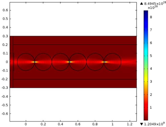
**Figure 5.** Linear waveguide arrangement formed with six LLs. The EM wave is guided through the linear network of lenses and the wave defocuses in the last lens. The result is in agreement with figure 1(ii). Additionally, the guiding is almost perfect since the losses are practically zero.
