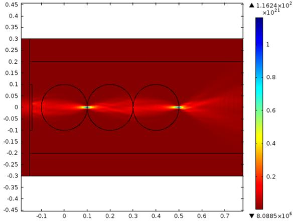
**Figure 9.** Linear waveguide arrangement formed by three lenses. We simulate the propagation of the EM wave including the Kerr effect. We can see that the focus points are located again on the surface of the lenses.
