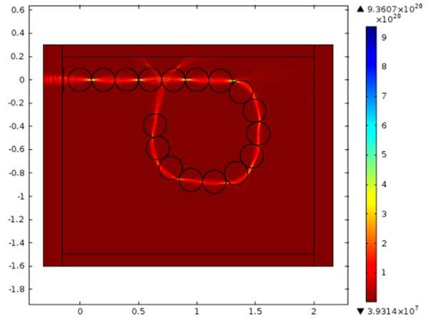
**Figure 7.** A full circle bend waveguide is formed by seventeen LLs. The EM wave is guided through a circular orbit. The losses in this arrangement are approximately 30% since  $E_{OUT}/E_{IN} = 0.70$ .
