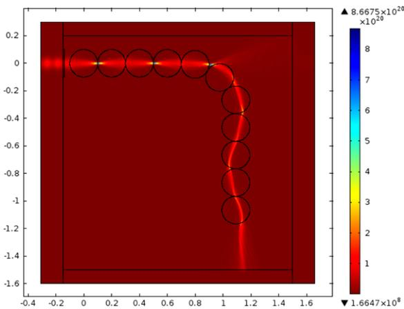
**Figure 6.** A right angle bend waveguide is formed by eleven LLs. The EM wave is guided and bends at a right angle through a network of lenses. The losses in this case are approximately 27% of the initial amplitude, i.e  $E_{OUT}/E_{IN} = 0.73$ .
