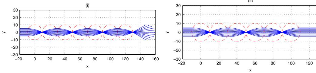
**Figure 1.** The red dotted lines denote the arrangement of lenses. The blue lines show the ray tracing. Light is guided by LLs across the linear network. (i) Arrangement with seven lenses (left figure). We can see that all rays are focused on the last lens. (ii) Arrangement with six lenses (right figure). All rays exit in the same mode as originally entered, i.e. parallel to the waveguide axis.
