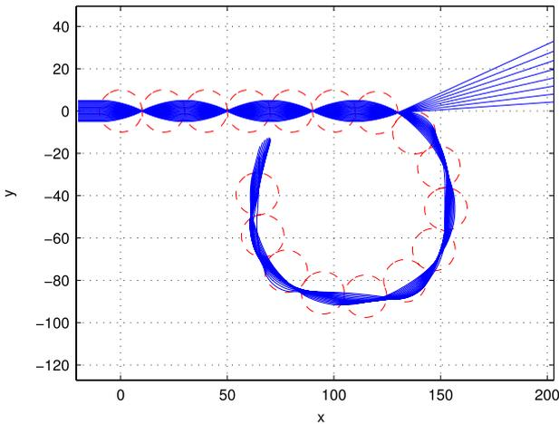
**Figure 3.** A full circle bend waveguide formed through seventeen LLs. The ray tracing is performed through the ray tracing methods. We see that Luneburg waveguides can guide light in a complete circle bend trajectory; more complex paths are also possible.
