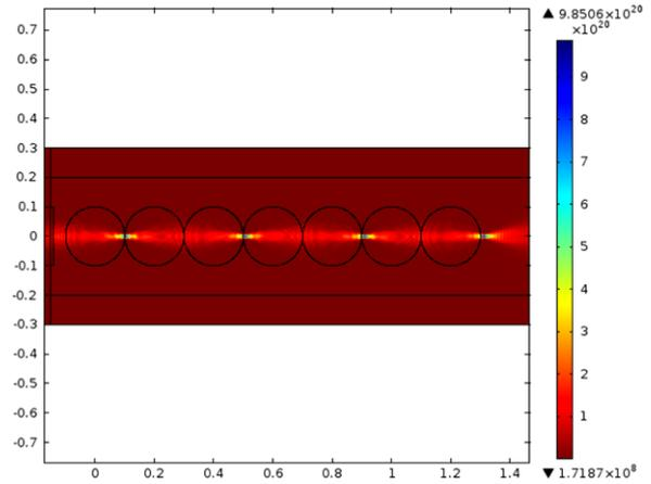
**Figure 4.** LLW arrangement with seven lenses. Beam guiding and focusing on the surface of the last lens is observed. The result is in agreement with figure 1(i). Furthermore, no losses are observed.
