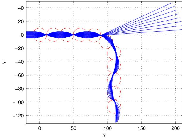
**Figure 2.** A right angle waveguide is formed through a network of eleven LLs. The ray tracing is performed analytically using equation (A.27). We observe efficient guiding with a total bend of  $90^\circ$ .
