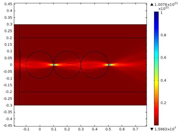
**Figure 8.** Linear waveguide arrangement formed by three lenses. We simulate the propagation of the EM wave without any nonlinearity (Kerr effect). We can see that the focus points are shifted out of the surface of the lenses.
